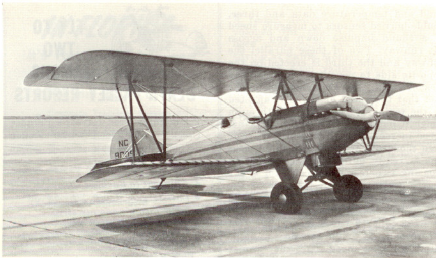
A Curtiss OX-5 powered this Travel Air 2000. Note overhanging counter-balanced ailerons
